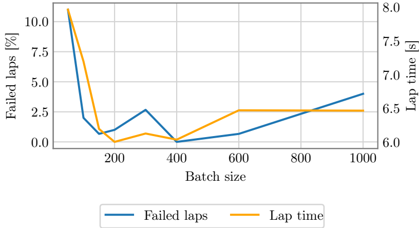
Figure 5.7: Percentage of failed laps and lap time under evaluation conditions of end-to-end agents with batch sizes from 50 to 1000. The percentage of failed laps is mapped onto the left vertical axis, while the lap time is mapped onto the right vertical axis.
