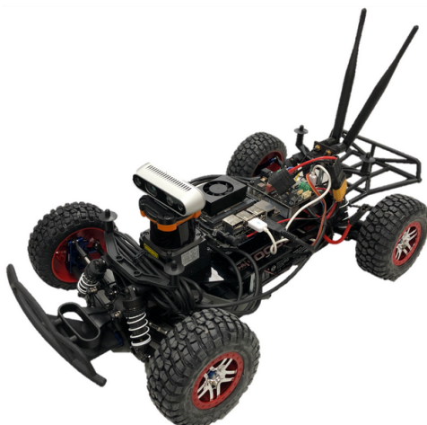
Figure 1.1: A standard F1tenth vehicle, built on the chassis of a miniature RC car [6].
