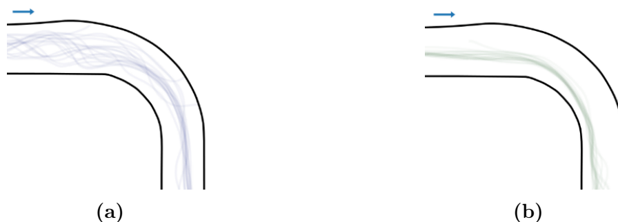
Figure 2.11: Distributions of paths taken by (a) an end-to-end and (b) a partial end-to-end agent to round a corner multiple times during an experiment by Ghignone et al. [14].
